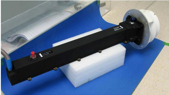
**Figure 1.** L-band TWT with an output power of 150 W in radiation cooled design
